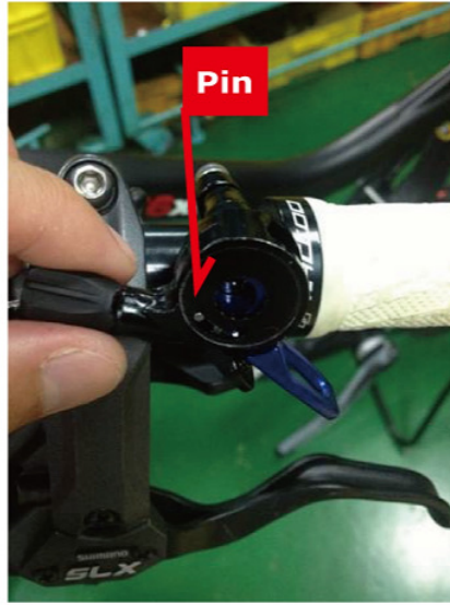
Be careful of the pin. If it falls out, the lockout will not function
