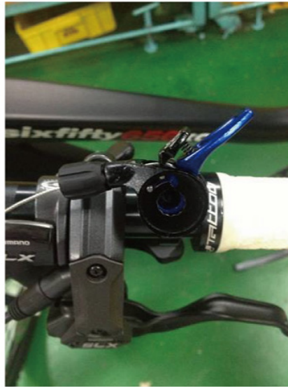
Position the lever to your personal preference then install back onto the mount.
