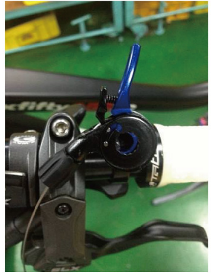
Position the lever to your personal preference then install back onto the mount.
