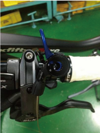
Position the lever to your personal preference then install back onto the mount.
